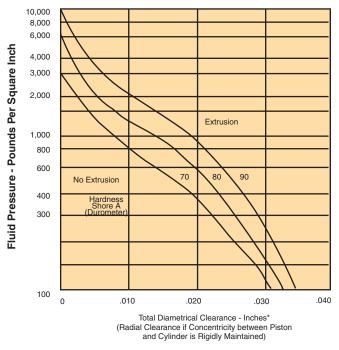
Extrusion-Pressure/ Hardness/Clearance-gap Relationships
